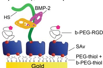
Figure 1: schematic representation of the biomimetic platforms that will be developed in this project.
